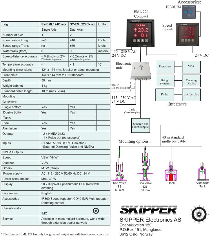
$\ast$  The Compact EML 124 has only Longitudinal output and will therefore only give that information within the NMEA outputs
