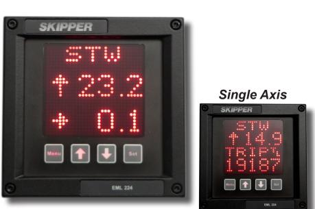
The SKIPPER COMPACT EML 224 is a single or dual axis speed log, working on the electromagnetic principle, providing longitudinal and transversal ship's speed relative to sea water. The COMPACT EML 224 gives accurate navigation parameters, measured as they happen, and presented in a logical, user friendly way.
